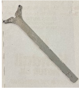
Crewe factory "slipper flywheel torque setting tool" for 1930s to Cloud III
