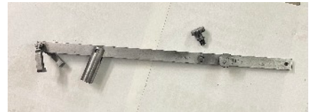
Crewe "crankshaft main bearing removal tool" Note the markings "BSF" (British Standard Fine) and "UNF" (Unified National Fine), which are different threads. Used for post-war 6 cylinder
