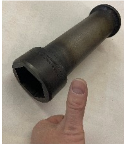
Hand-fabricated "6-point extra deep socket" used to compress and decompress coil springs from early post-war through Cloud III
