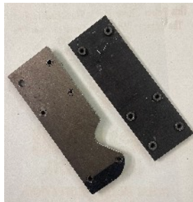
Hand-fabricated jig to remove stubborn or broken studs on exhaust manifold for post-war 6 cylinders. Hardened carbide bushings will help to find the exact center of the problem stud. Then, extra drilling for drill-tap size. The curved notch goes around the power steering pump if fitted.
